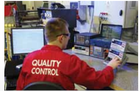
Final test of actual duty cycle, electrical safety, EMC
